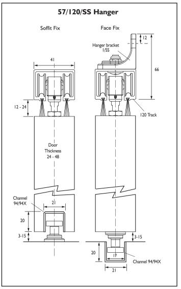
For MDF doors 19-23mm you must use hanger 52/120/SS and for doors 24-48 there is an option of surface mounted or routed (51/120/SS or 57/120/SS)
