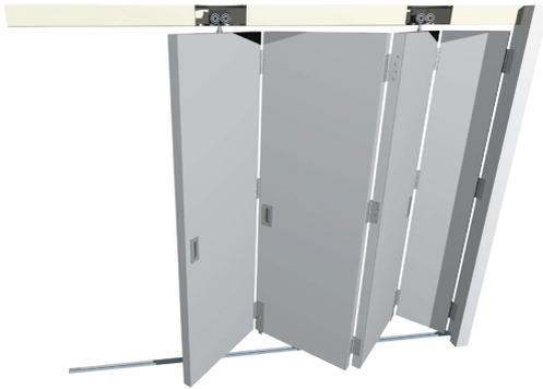
Specifically developed for commercial applications requiring heavyweight, top hung, central folding wooden partition doors. Doors are hung centrally and can fold to one or both sides. For applications hinged to the jam 3.5, 5.5 or 7.5 doors can be used with the half door hinged to the jam. For best operation of floating units, 5, 7 or 9 doors should be used. Any access doors should be hinged separately to the jamb.
