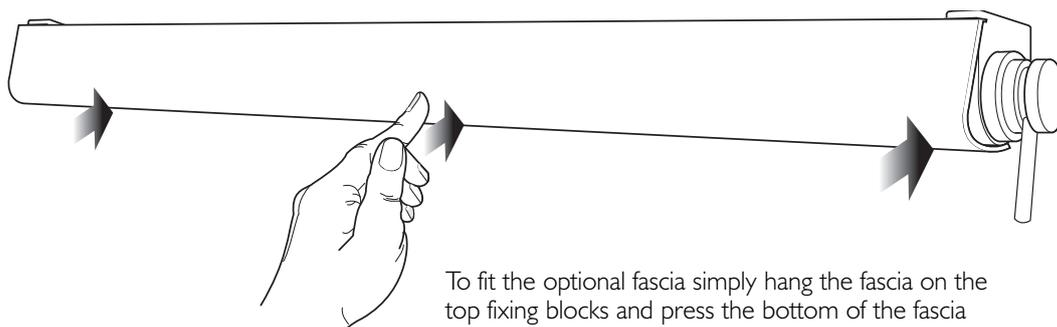
To fit the optional fascia simply hang the fascia on the top fixing blocks and press the bottom of the fascia until it clicks into position.
