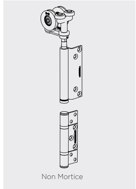
P C Henderson offer a choice of three different hinge options in the Securefold range, this enables us to offer our customers a choice in the look and feel of their project as well as variances on the preferred method of installation and door material. Please note for Securefold 150 and Securefold Ultra, mortice standard hinges must be used.
