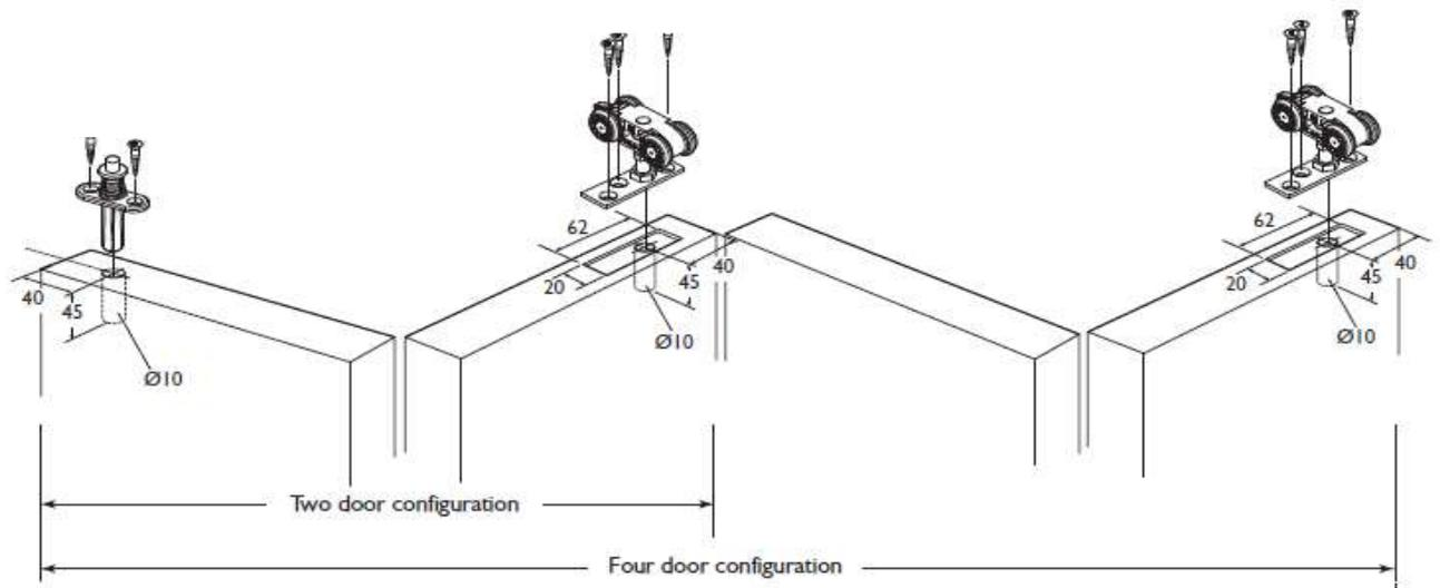
**STEP 4:** Position and secure the bottom pivot body to the bottom of the pivot door.
