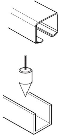
**STEP 12:** Route guide channel into floor and secure into position.
