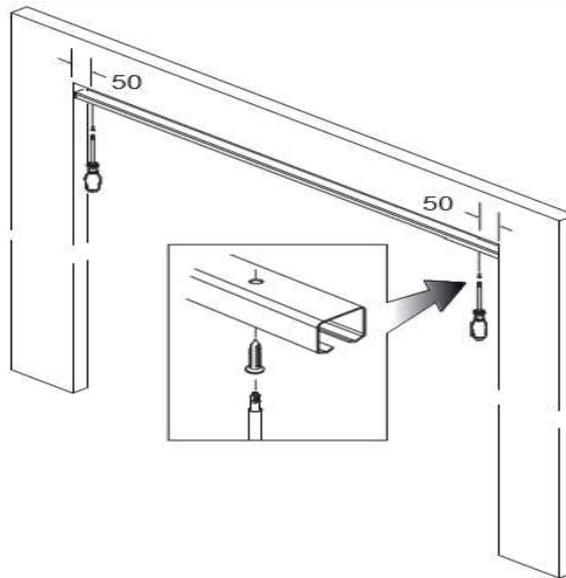
**STEP 10:** Use a plum line to align hole centre for the top pivot to the bottom pivot plate and screw into place - this should be 46mm from the door frame.
