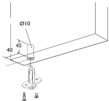
**STEP 5:** Attach guide to bottom of the doors (HF40 kits only)
