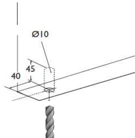
**STEP 2:** Position and secure top pivot body to the top of the pivot door
