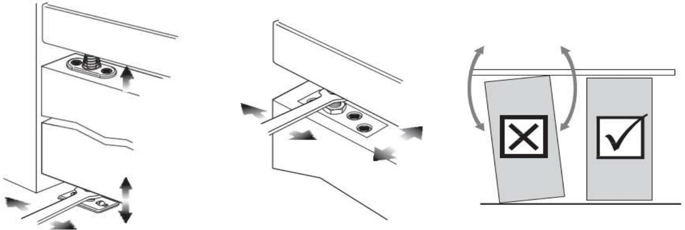
**NOTE:** When adjusting, ensure that the hanger supports the weight of the doors along with the whole length of the track.
