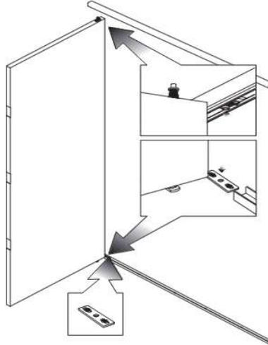
**STEP 15:** Adjust door height using spanners - use 13mm spanner on pivot door and 10mm spanner on hanger door
