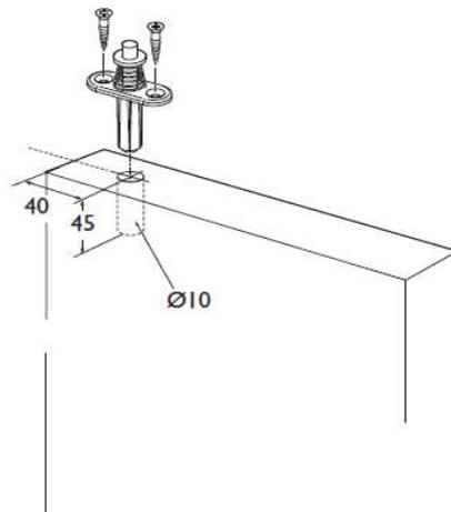
**STEP 3:** Fit hangers to doors - for 2 door applications fit hanger to 2nd door. For 4 door applications, fit hangers to 2nd and 4th doors.
