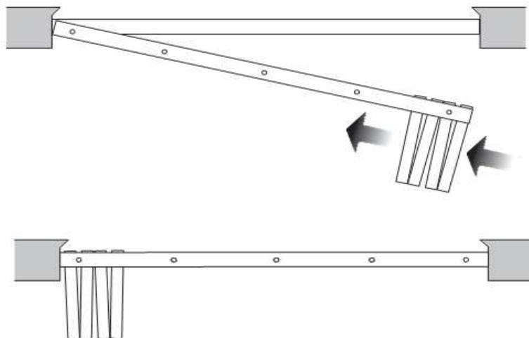
**STEP 14:** Locate the bottom pivot and top pivot onto the plate
