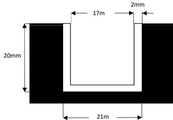
It is the installer's responsibility to ensure the guide channel has been routed and secured into the floor appropriately.
