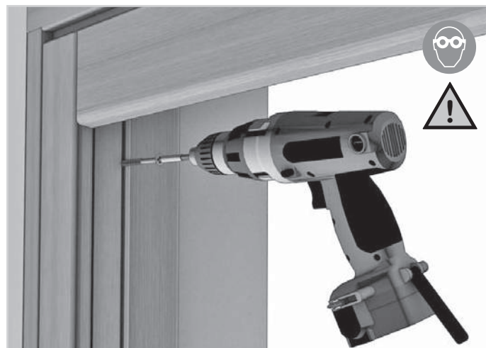
68. Secure with 6x120 screws if the height of the profile is 100 mm, 6x140 if the height of the profile is 110 mm.
