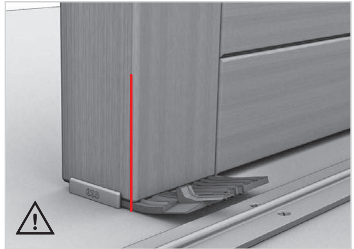
74. Insert the pad aligning the side of the pad flush with the fixed sash.
