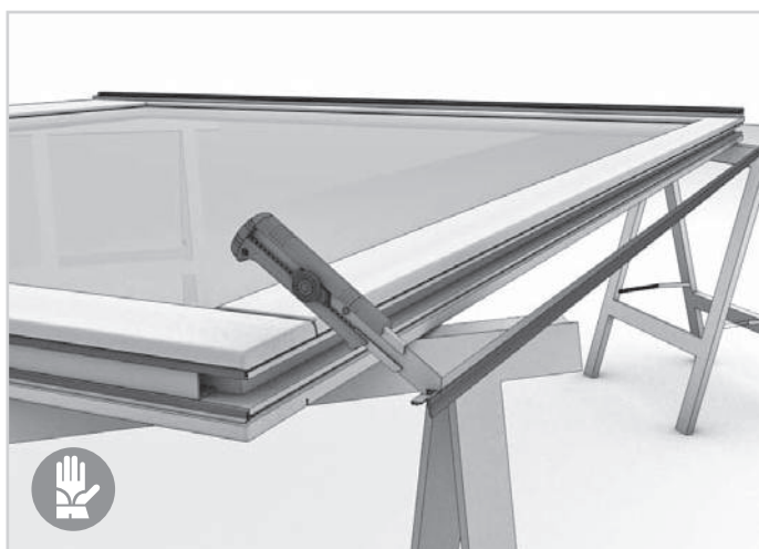
95. Cut the top gaskets for the sliding sash to size, taking care to shape them to match the front part.
