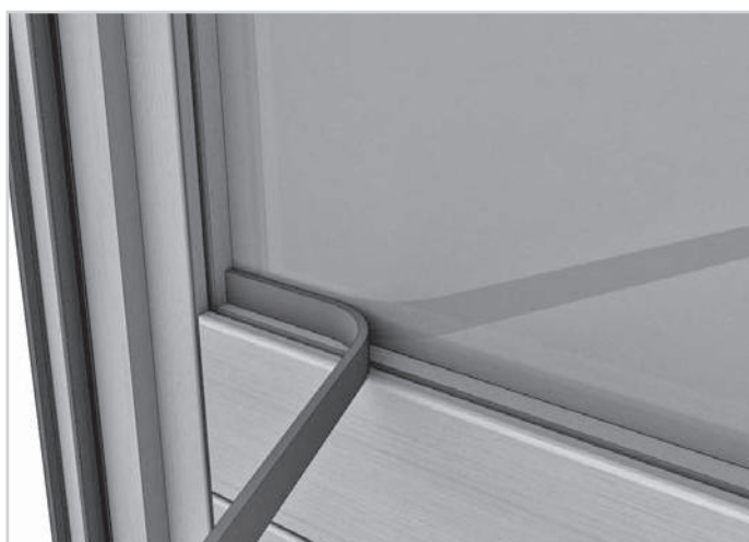
83. To improve sound insulation, you should use a special gasket for the glazing bead also internally. Alternatively, silicone the inner part of the glazing bead against the glazing.
