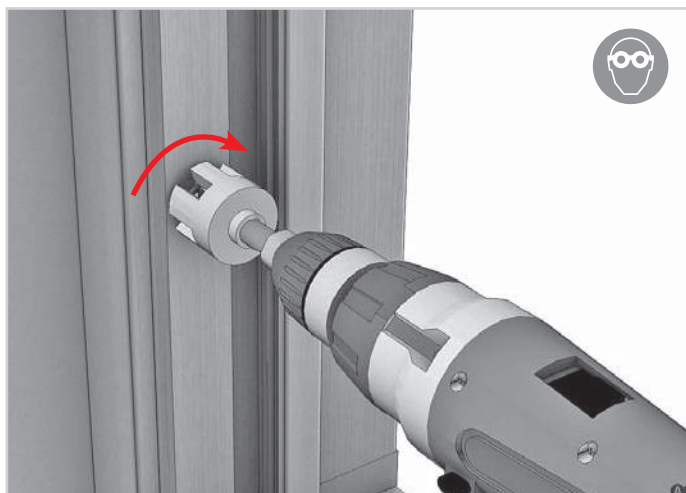
109. Tighten until reaching the end position.
