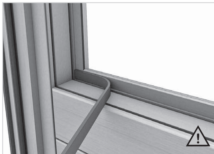
80. Apply gasket tape to the outside edge of the glazing bead profile around the perimeter of the sash.
