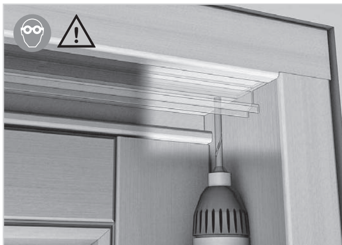
115. Drill holes in the head jamb with an \varnothing 8 drill bit for housing the bumpers.
