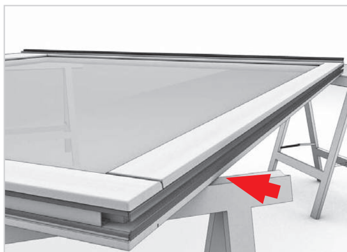
96. Insert them in the milled sections provided in the top rail.
