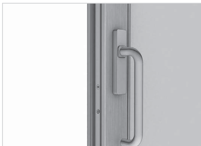
114. Slide the finish plate in the lever until it overlaps the closure.
