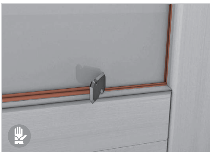
89. Remove the excess sealant using a spatula.
