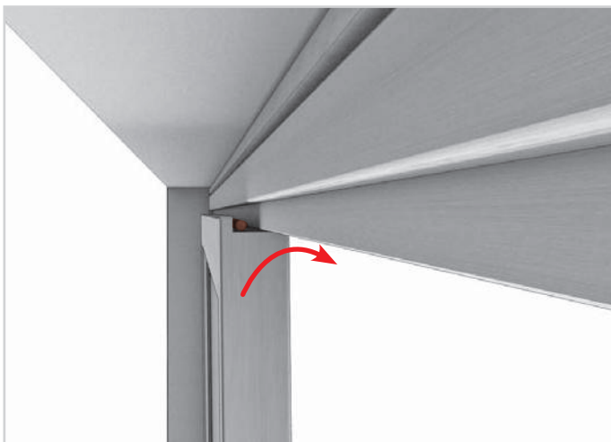
63. Turn the sash until it is snug against the head jamb.
