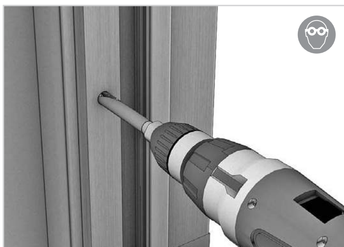
107. Drill a hole using an \varnothing 10 drill bit for softwood or \varnothing 11 drill bit for hardwood.
