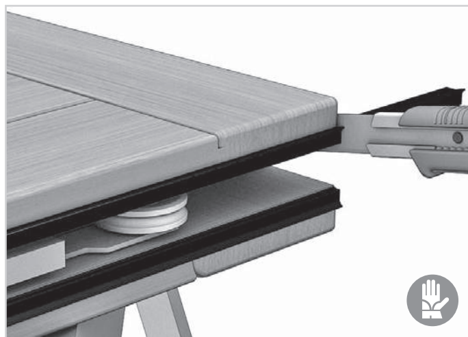
44. Cut off the excess parts at the end.
