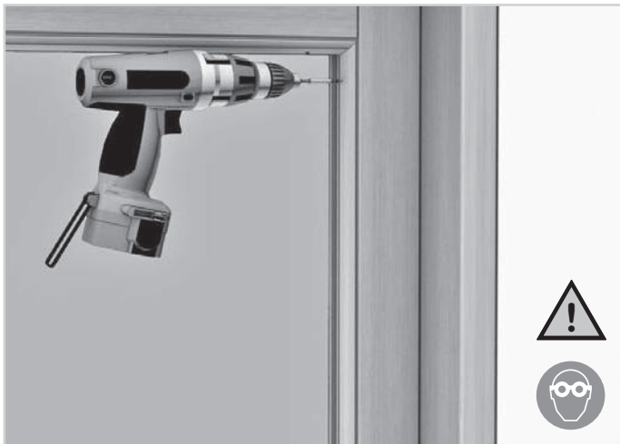
85. Secure the glazing bead with \varnothing 3x40 screws diagonally.
