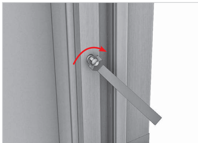
110. Use a spanner to adjust the position of the pin.
