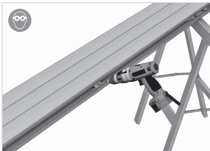
37. Insert and fasten the carriage link rod guide pad to the middle point of the sash.
