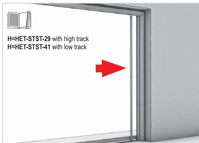
30. Insert the pin holder profile previously cut according to the instructions provided in the technical manual.
