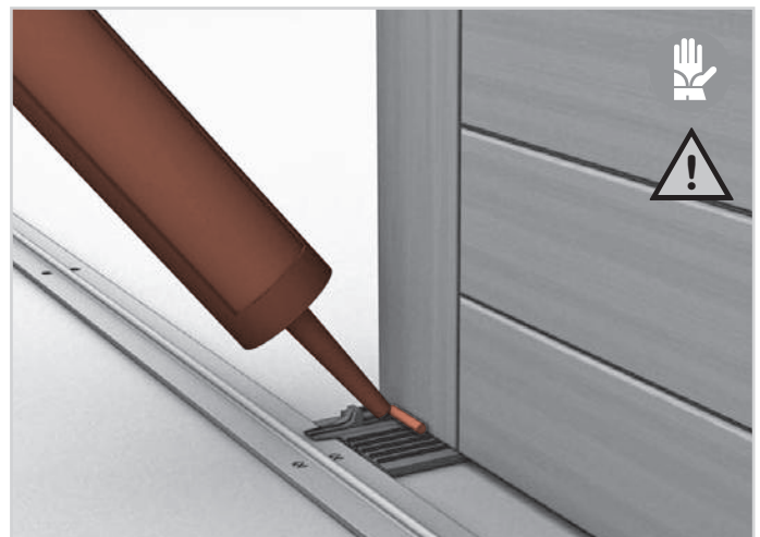
76. Silicone contact point above the pad between the gasket retainer listel and fixed sash.
