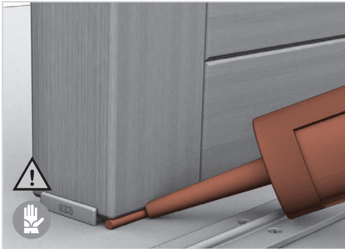
73. Apply silicone along the edge between the supporting profile and bottom pad.
