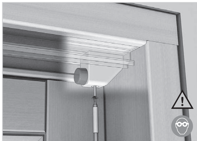
116. Insert the bumpers and tighten using the screws provided in the kit.
