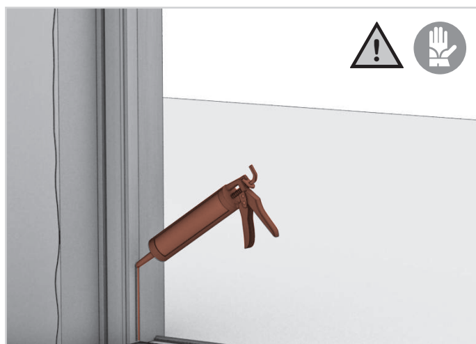
60. Apply silicone along the entire length of the fixed sash listel.
