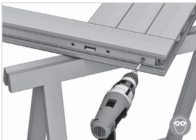
39. Secure the lock starting from the connecting screw with the front carriage.
