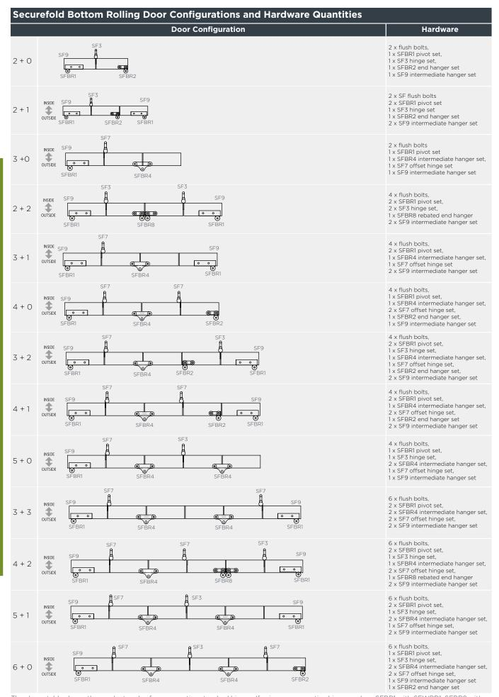
The above table shows the product codes for our mortice standard hinges. If using a non mortice hinge, replace SFBR1 with SFWBR1, SFBR2 with SFWBR2, SFWBR4 with SFWBR4 and SFBR8 with SFWBR8.
