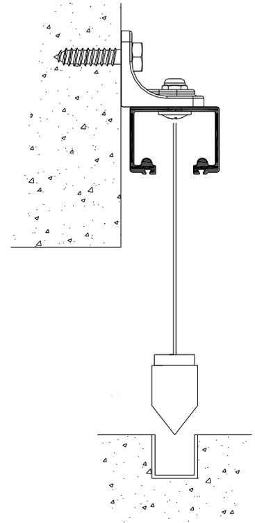
It is the installer responsibility to ensure that the correct fixing/wall insert is used and is suitable - depending on the wall/ceiling/floor type and quality
