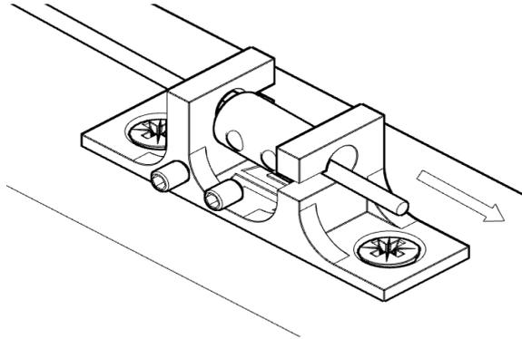
**Step 10:** Set the door closing mechanism to suit requirements of speed.
