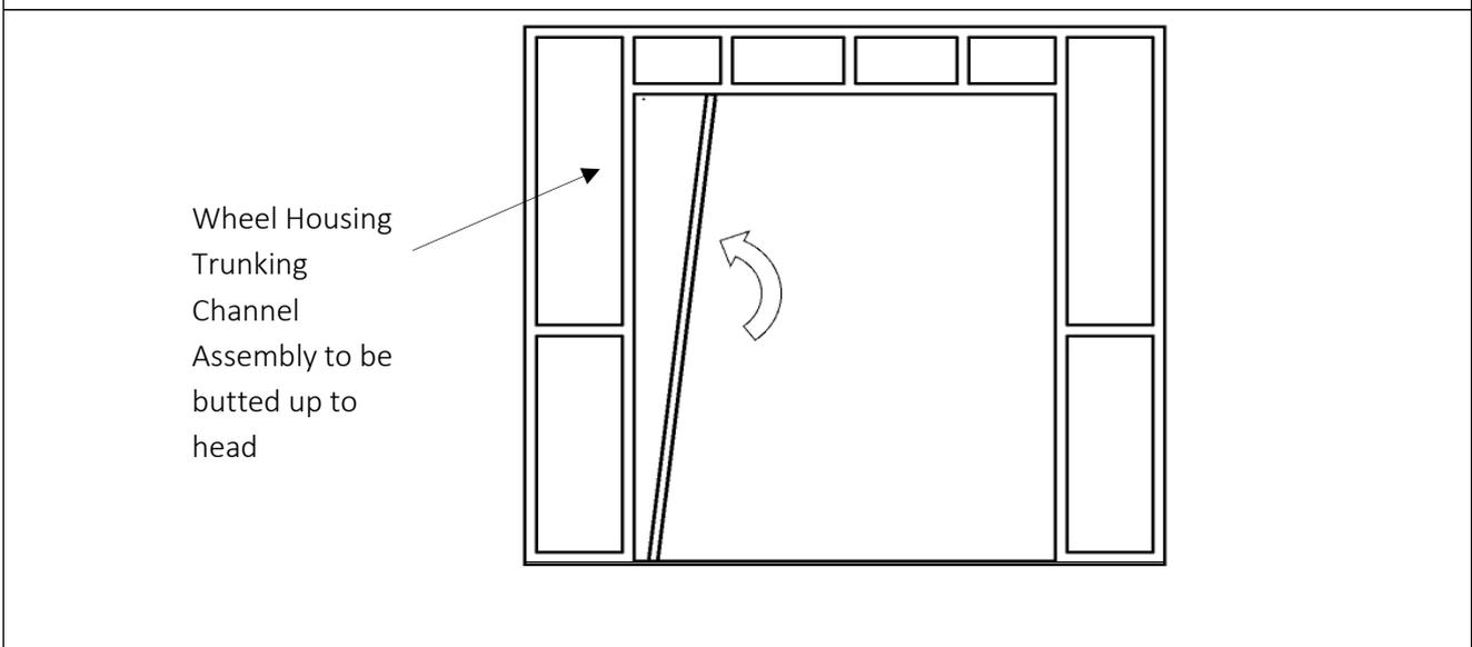
**Step 5:** Secure wheel housing trunking channel assembly to jamb upright using screw D.
