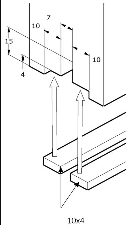
**Step 12:** Cut track packer to suit opening and secure with screw C (pilot drill & countersink if required)
