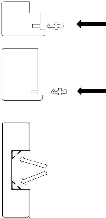
**11B:** Add intumescent strips and acoustic seal to fire rated liner kit
