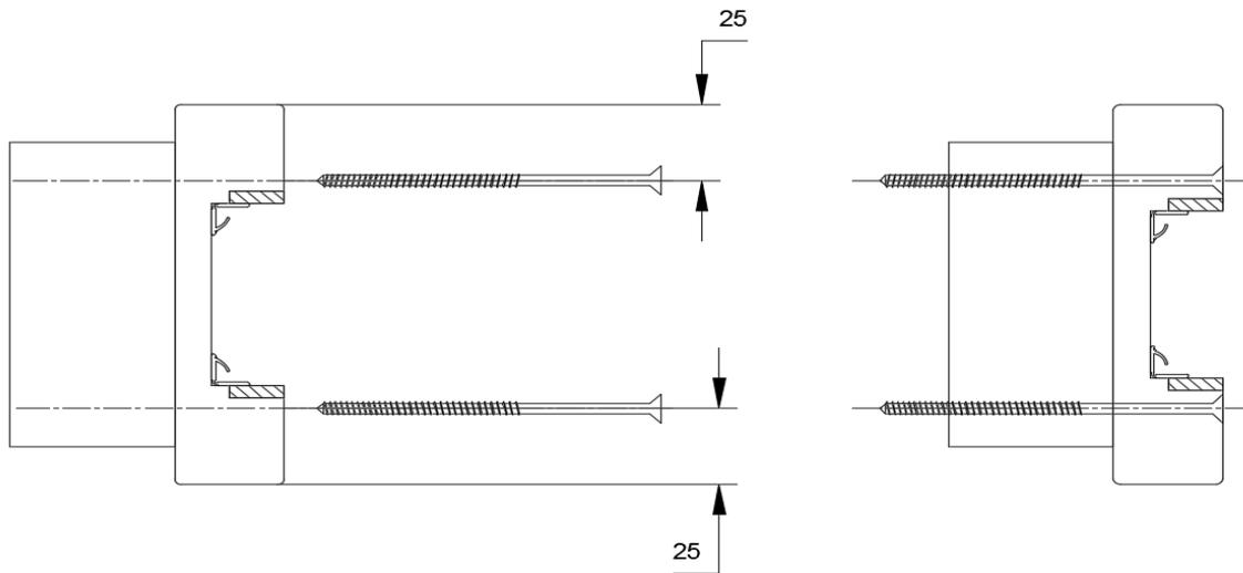
**STEP 15b:** For use of liner kit for self-closing mechanism; cut down jamb upright to suit opening and secure with Screw B (pilot drill & countersink if required)
