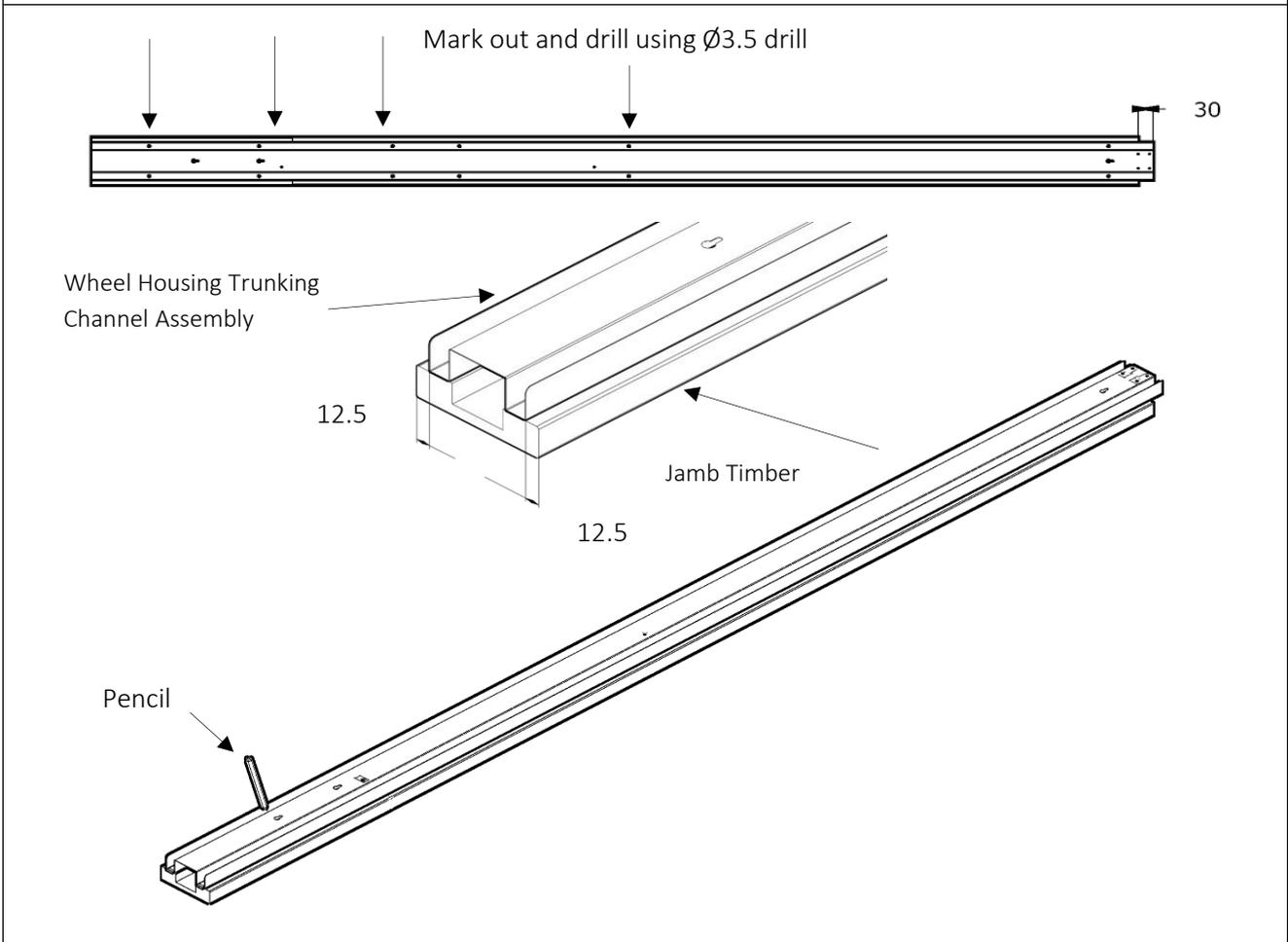
**Step 4:** Position wheel trunking channel assembly into opening.
