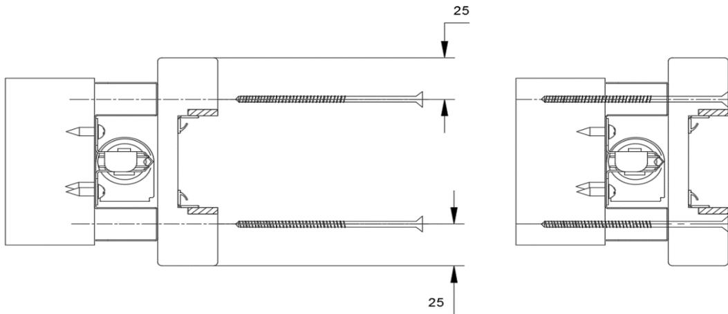
**Step 16:** Cut header into two pieces using the below calculation and secure with screw C (pilot drill & countersink if required).
