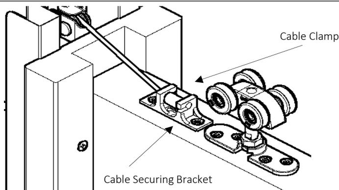
**Step 9:** With door in fully closed position, loosen grub screws in the cable clamp and pull cable through the clamp to apply tension to the cable, adjusting length of the cable to suit the travel of door width.
