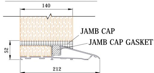
ALTERNATIVE ALUMINIUM THRESHOLD COMES COMPLETE WITH 94P AND ENDCAPS AND IS PREDRILLED FOR DRAINAGE
